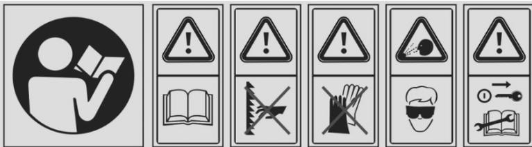
The safety signs (pictogram) are positioned on the machine and signal the various hazardous situations. **Keep them clean and replace them should they come away or are illegible or damaged.**
