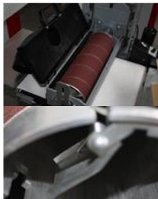
First open the cover, which is fastened with a screw. The clamping lever on both sides allows the end of the abrasive sanding belt to be unthreaded and the entire cylinder to be unwound. The other end of the abrasive sanding belt can also be released by this lever.
