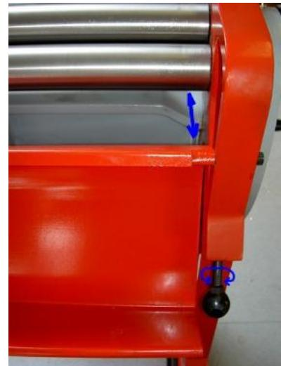
To remove the front upper roll turn the thumb screw by 90° and unscrew the clamp screws.
