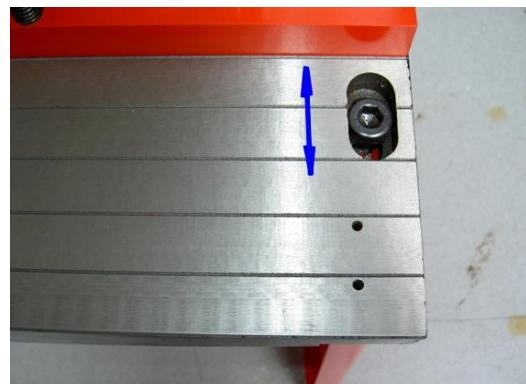
For bending the different segments can be removed or replaced, depending on workpiece size, so that a defined bending edge can be generated. For this purpose, loosen the screw of the corresponding segment to move or remove this. After new setting retighten the screw.
