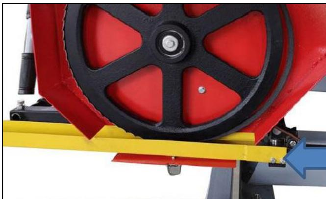
Ensure the blade support arm is locked into place after tensioning the blade.
